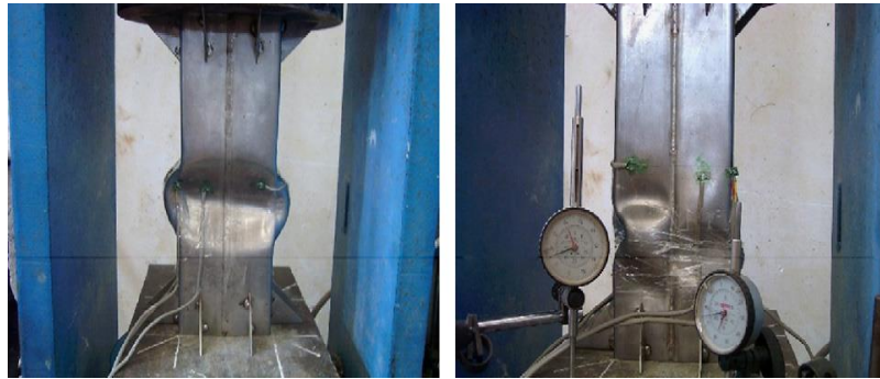
Fig.8. Deformed shape of square hollow section.
